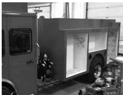
The body and pump mounted to the chassis.
